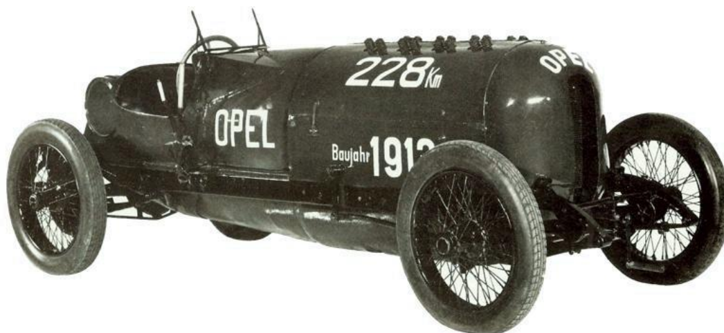
A 1913 12-litre racing Opel with 16 valve 4-cylinder engine
